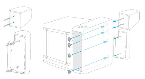
1. Screw the short ends of the bolts into the holes in the underside of the wings and armrest pads.
